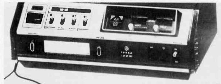
**GE's** **TA640** 8-track tape deck, retailing for \$219.95, plays all 4-channel pre-recorded tapes through 2-channel system. Among other features are two microphones and a one/all switch to allow recording on one track or all four in sequence.
