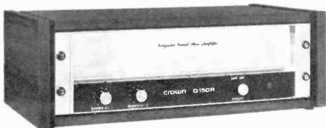
▲ **CROWN D-150A** power amp has rating of 80 watts RMS per channel, unique rear panel stereo-mono switch, two direct-coupled amp circuits.
