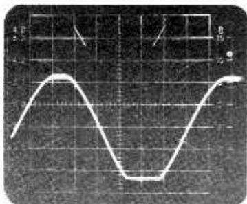
When a typical transistorized amplifier tries to deliver more power than it can the top and bottom edges of the waveform clip sharply and abruptly and not always symmetrically. Result: high-order harmonic distortion, raspy and irritating.
