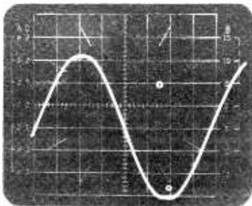
When a tube amplifier such as the Luxman MB-3045 is driven into overload, the clipping is softer with more rounded edges to the waveform. The resulting distortion is much less audibly bothersome.
