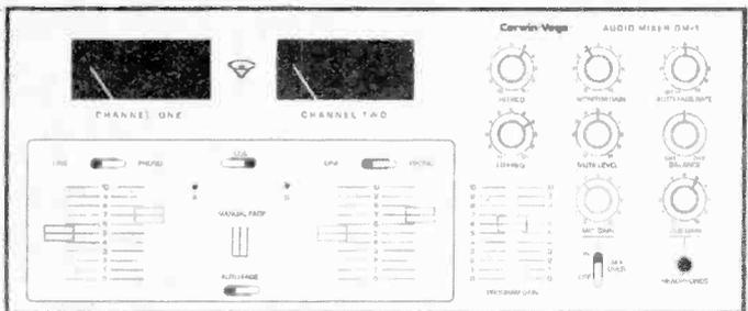
CERWIN-VEGA DM-1 disco mixer has Autofade circuit that crossfades between two stereo program sources, talkover switch, cue circuit.
