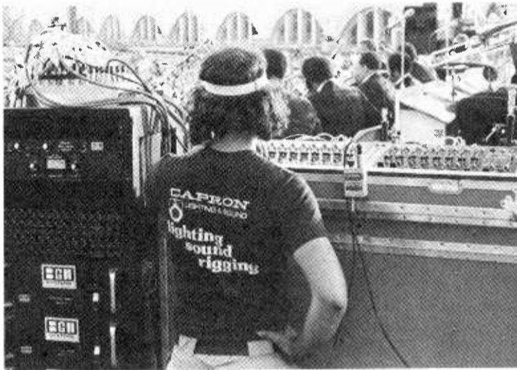
Capron monitor mixer Al Kennedy checks out system during a pre-show run-through. Visible are the UniSync Trouper I mixer, in its road case, and some of the BGW power amps used in monitor and house setups.
