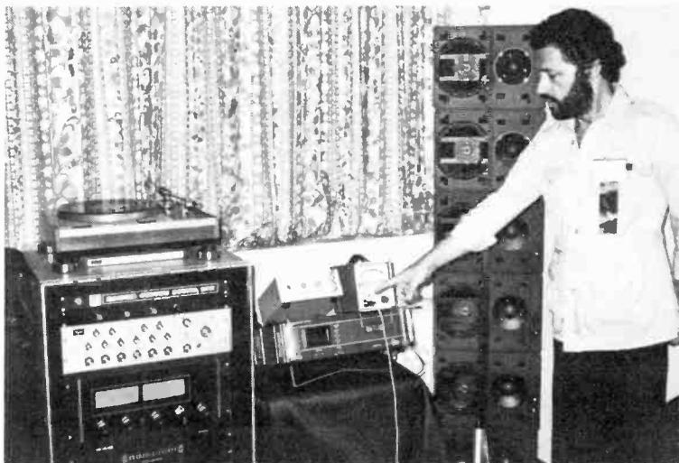
ROSNER Custom Sound's Alex Rosner "equalizes" room with real-time frequency response analyzer, calibrated mike to a sound level meter, using Philips bi-amped 944 speakers.
