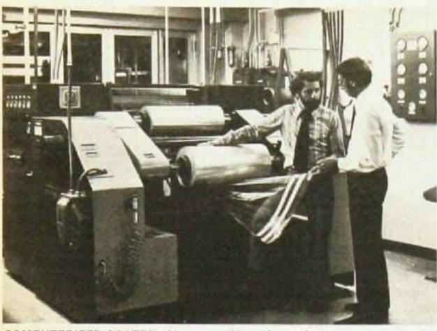
COMPUTERIZED COATER—Memorex (Santa Clara, Calif.) plant's expansion includes this state of the art computer controlled audiotape coating line, being inspected by Chuck Levdar, left, plant manager, and Howard Earhart, audio division general manager. The clear polyester is unwound, coated and passed through a series of ovens before being "polished" and slit into cassette, 8-track or open-reel products.
