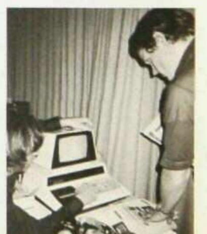
**EVENTIDE** Clockworks' Rich Factor, left, shows firm's spectrum analyzer display on PET home computer to Tom Brightwell, Phoenix Civic Plaza. Eventide circuit makes the computer function as a real-time third-octave spectrum analyzer.
