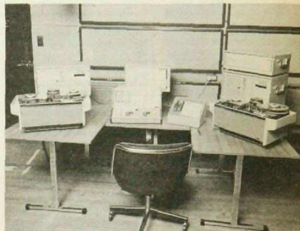
Edit Console: Electronic "splices" are accomplished on modified video editor, center, with finished edits transferred to recorder, right. Right is the complete two-track digital system comprising IVC video recorder, Decca digital processor, and Decca outboard analog-digital converter, top.
