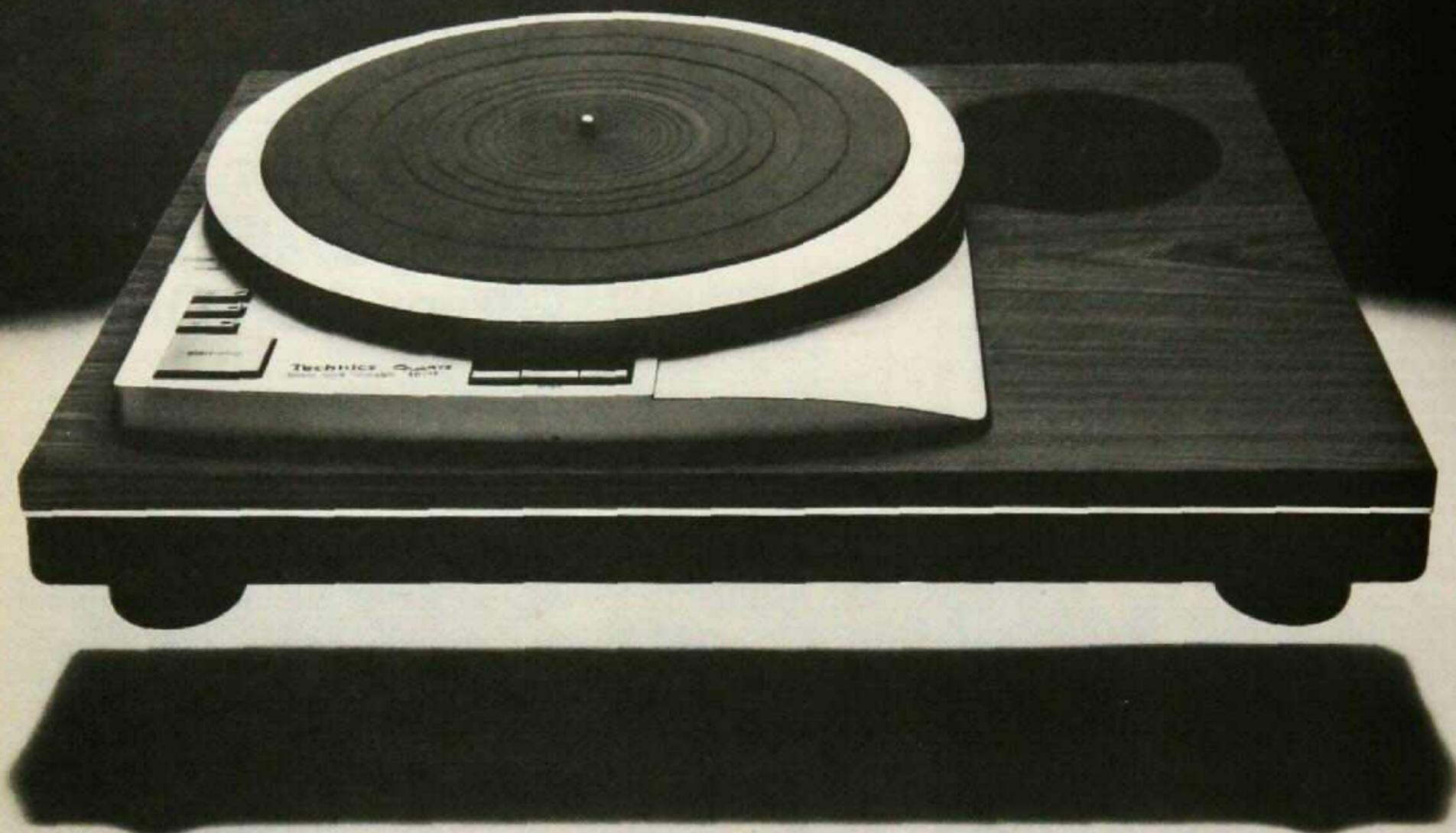
You know what made the SP-10 MK2 our best turntable, and why so many radio stations use it: Wow and Flutter of 0.025% WRMS. Rumble of -78dB (DIN B). Speed accuracy within an astonishing 0.002%. And amazingly high torque for a start-up time of 0.25 second.
