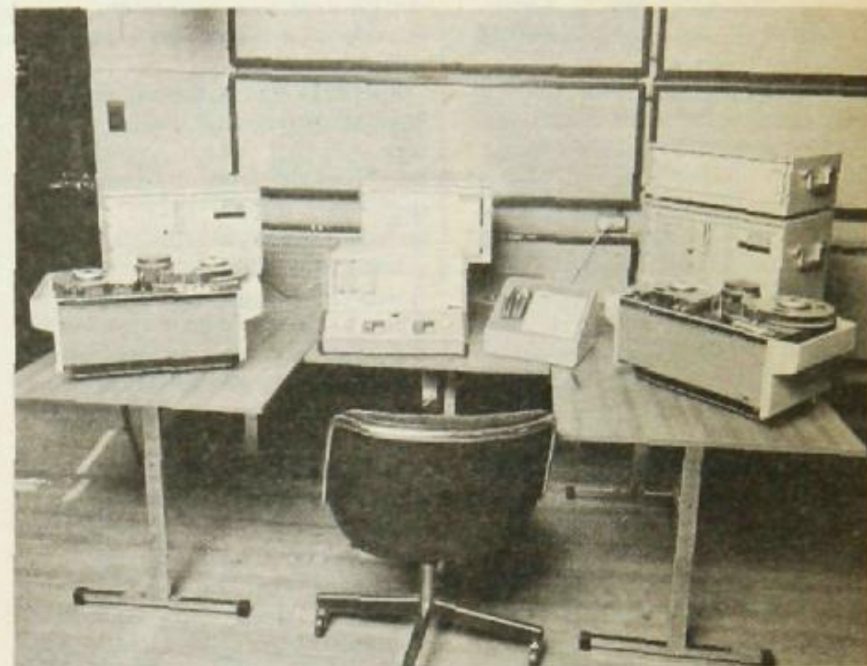
Edit Console: Electronic "splices" are accomplished on modified video editor, center, with finished edits transferred to recorder, right. Right is the complete two-track digital system comprising IVC video recorder, Decca digital p.p.s.s., and Decca outboard analog-digital converter, top.
