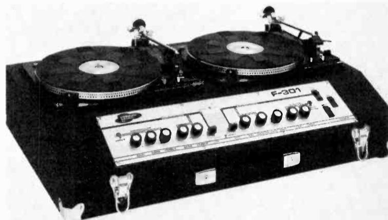
**DISCO CONSOLE**—This Farallane disco console features low noise integrated circuits, has harmonic distortion of less than 0.3% and a frequency response of 50Hz to 38kHz minus 3dB. The unit utilizes BSR model C206 belt driven turntables with strobe and pitch controls, viscous damped cueing, speed and anti-skate controls. It sells for \$775.
