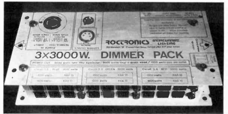
**DIMMER PACK**—Roctronics Entertainment Lighting has developed a dimmer pack unit for use in discotheques and other nightclubs. The unit, weighing 15 pounds, features three 3000 watt dimmers, 18 grounded outlets, six fuses, spare fuse and holder, detachable power input connector or direct-wired electrical box, remote control input, remote slave output, two live power outlets, rubber bumpers, guard flanges, and C-clamp and wall mounting holes. It comes with a three-year guarantee.
