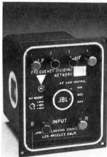
**FREQUENCY DIVIDER**—The James B. Lansing Sound Co., has introduced three new Frequency Dividing Networks as part of its Professional Series. The units, models 3110A, 3115A and 3120A are equipped with a three-position high frequency equalization boost switch which is said to compensate for power response roll-off. According to JBL engineers the design allows the networks to be utilized in systems incorporating the company's exclusive line of Bi-Radial Constant Coverage horns.
