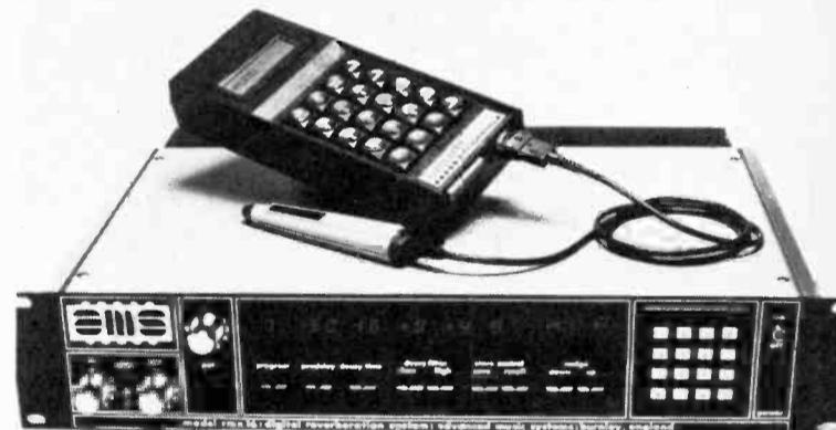
**ADVANCE REVERB**—This model RMX-16 is a 2U 19 inch rack mount system on an 18kHz bandwidth, offering nine programs of reverberation ranging from the smallest room to the largest hall. Once the program is selected, the user controls the delay time. Pre-reverberation delay can be added, and independent adjustment of both high and low frequency decay characteristics is possible.
