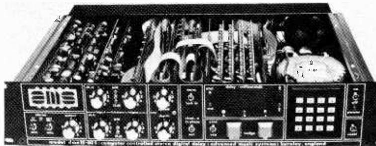
**DIGITAL STEREO**—Advanced Music Systems has introduced the model DMX 15-80S stereo digital delay line with maximum delay capability of 33 seconds at 18kHz bandwidth. Mono or dual pitch changers are optional.
