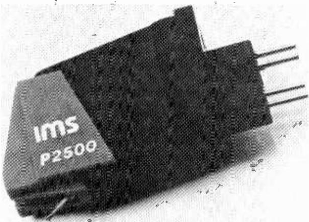
The P2500 from the Nagatronics Corp. in Freeport, N.Y. is one of two new P-Mount induced magnet phono cartridges. It features a diamond elliptical stylus in a low mass cantilever with a non-aging high energy samarium cobalt magnetic activator.
