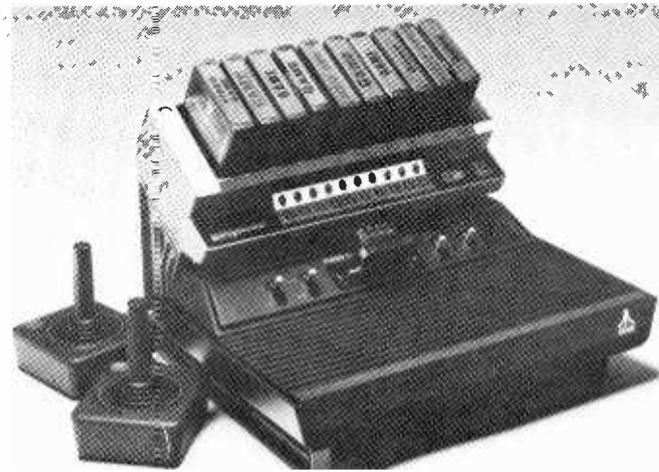
The RomScanner from MarJac Technology of Glendale, Wis., holds 10 Atari 2600 Series VCR cartridges that can be changed instantly by pushing numbered buttons on the control panel.
