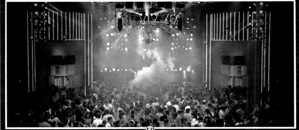
Capacity: 2300 - Box office complete with three computerized cashier stations for ticket sales (advance capability) - Three diessing rooms complete with full bath - Stage dimensions: 20'd, 30'w, 4'h - Proscenium height: 25' - Fly grid height: 55' - Power: 100 amp, 3 phase - House Sound: Richard Long Associates - House Lighting: See Factor, Inc. - Additional tech information available upon request
