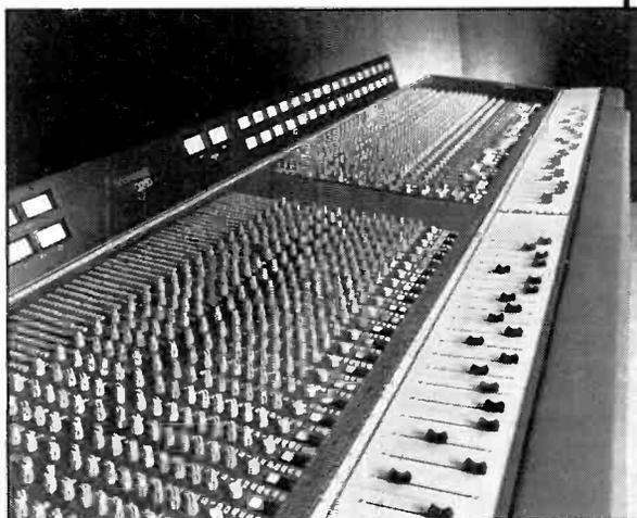
Soundcraft 3200 Console with 36 inputs and full 32 buss routing.
