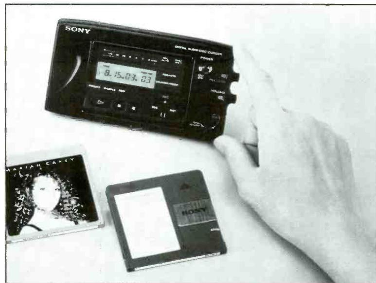
A prototype of a Sony mini disc player/recorder unit, with blank disc
