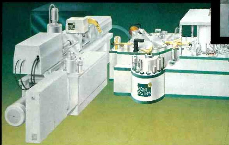
With a cycle time of 3.0 seconds per CD the **RONDO-LINE** is the world's fastest replication-system for 120 mm CD's, as well as for Mini-Discs.
