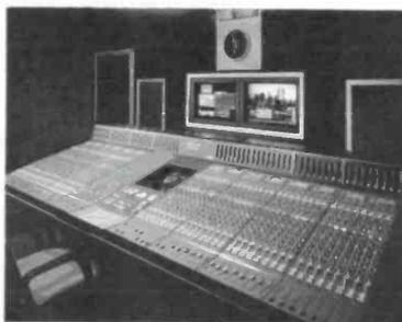
Solid State Logic's Axiom Digital board, the company's first foray into the digital recording, mixing, and editing.
