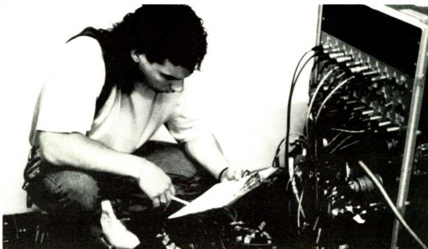
Good notations and labelling are necessary when patching cables for live recording.
