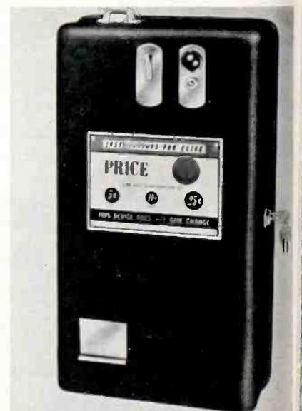
NRI has designed a new coinage unit (CB June 20) Model 10-18-000 series for coin-op car washers. Unit accepts nickels, dimes, quarters in any combination to maximum \$1.50. Vends at single settable price or multiple prices to allow for variety of rates in line with promotions, weekend rates, etc. Details appeared in June 20 Cash Box.
