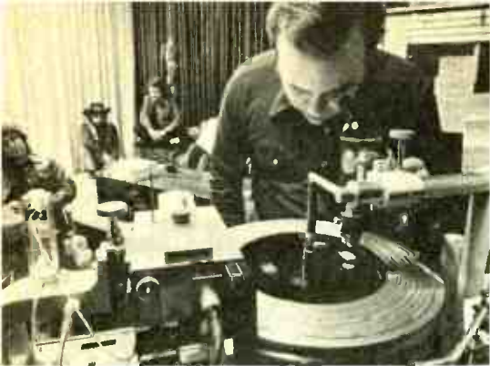
The final step: Engineer Mac Evans of Mustronics, Inc. works the lathe which cuts an acetate master from the finished 16-track tape.
