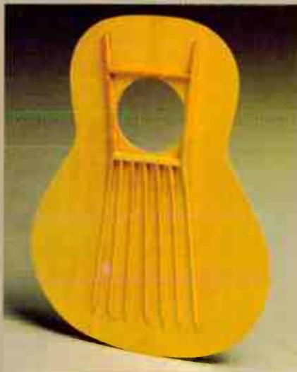
The Ovation A-brace. Seven carefully shaped supports run with the top grain instead of against it. A slight arch gives the top strength to resist changes in humidity.
