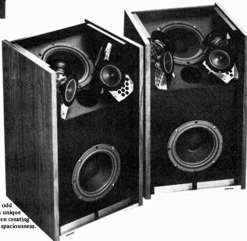
Four tweeters firing sound at odd angles give the Bose 601 a unique sound projection pattern creating an impression of spaciousness.
