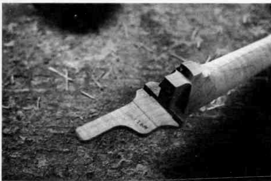
The joint where the neck fits the body must be hand-fitted.
