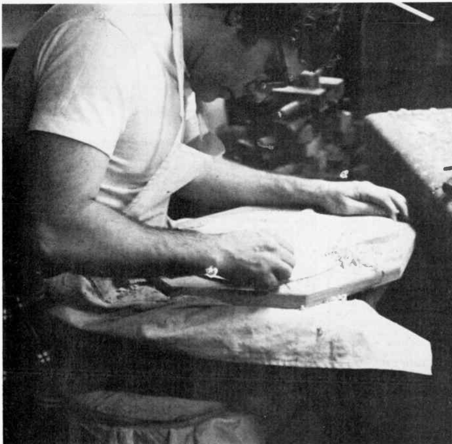
The top and back of the Gibson F-5 mandolin are hand-carved. If they are not perfect, they go straight to the scrap-heap.
