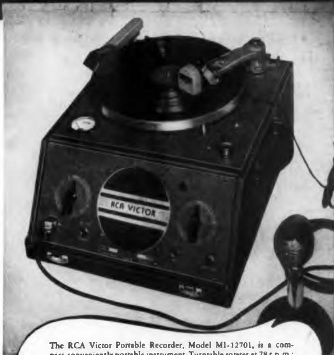
The RCA Victor Portable Recorder, Model M1-12701, is a compact, conveniently portable instrument. Turntable rotates at 78 r.p.m.; and will accommodate discs of from 6" to 12" in diameter. Immediately plays back finished recordings or other records. High fidelity throughout, this recorder also provides higher fidelity reproduction of Victor Red Seal and Black Label Records. Complete with RCA Aerodynamic Microphone and table stand. **\$179\***
