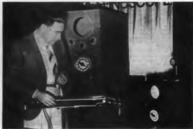
Engineer Lester B. Holmes looks over one of his new inventions, the Resonoscope, which checks the accuracy of all instruments and voice by science.
