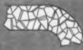
Diagrammatic drawing of cross section of ordinary brass, illustrating how crystal structure is irregular and hodge-podge. Note also how large the crystals are compared with Coprion crystals.
