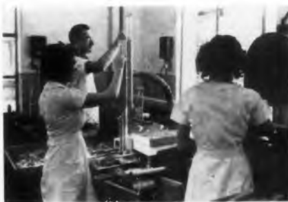
This picture shows some of those special reed cutters that I designed for making my reeds.
