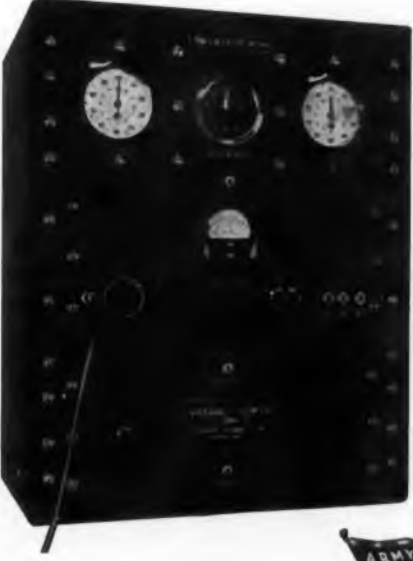
Above: Supercharger Tachometer, which measures speed of rotating parts from 20 to 33,280 c.p.m. Created for AAF, Wright Field, by C. G. CONN LTD., pioneer in sound and electronics research.
