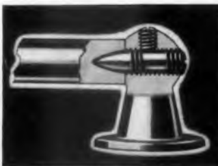
Quick, permanent key adjustment on all Conn wood clarinets. Patented adjustable pivot screw turns in or out for proper key hinge adjustment, then locks in place with set screw.
