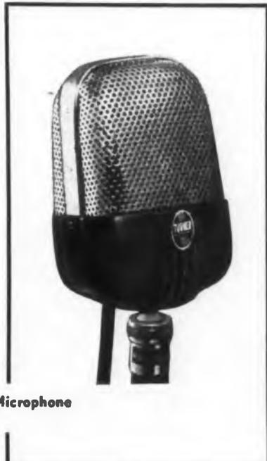
A great new microphone, designed especially for broadcast and recording where highest quality reproduction is desired. The Model 87 brings world famous Turner dependability to the velocity microphone field. Engineered with single element ribbon supported in high quality Alnico V magnet for maximum sensitivity. Shielding excludes hum pickups.
