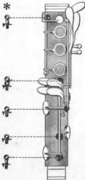
In ordinary clarinets, playing tends to loosen posts, shift key alignments, jam the action. That can't happen in this MARTIN FRERES #1. Each spring-tension post is first tightly threaded into place on the clarinet body. Then, to keep it swivel-proof for all time, a screw is sunk through the post deep into the wood. These ANCHORED POSTS will keep the action free-moving, the keys keenly responsive.
