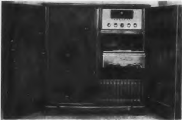
NEWLY INTRODUCED Admiral high fidelity combination has AM and FM radio and professional type record changer. Utilizing 20 tubes, a two way, dual-speaker installation, power amplifier, and record equalization system, the instrument is said to reproduce the full range of tones from 30 to 16,000 cycles.
