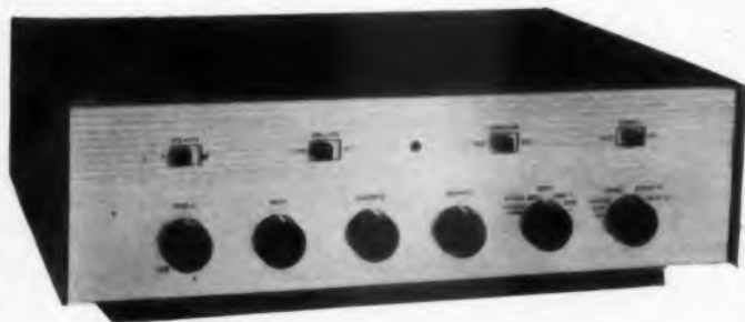
The Harmon-Kardon Tri-Plex Stereo Amplifier, Model A-224, provides peak efficiency in a compact unit. Included are controls for balance, treble, base, loudness, monaural-stereo, contour and rumble.
