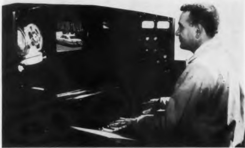
Raymond Scott isn't lazy; he's ingenious. The elaborate piano he's playing and watching is known as a Videola. It enables Scott to compose sound track music while watching the film involved. The film, projected on a movie editing viewer in another room is picked up on closed circuit TV and transmitted to the receiver in the Videola. A tape recorder and speaker system further enable Scott to keep track of the film and the sound track. A report that Scott may form the first Videola quartet has not been confirmed.
