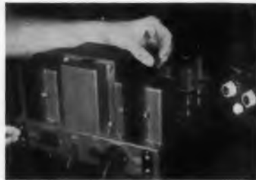
The two chassis Leak stereo amplifier is being set up here. Hand shows plug atop output transformer about to be plugged in to select proper value for particular speaker in this system. Index finger (lower left) points to terminal strip to which speaker wires are to be connected. At right is seen separate preamp-control unit.
