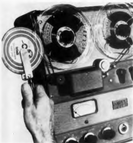
A stroboscope (speed checker) for testing tape recorders, this Irish Tape device checks the speed of any tape recorder at 3¼", 7½" or 15" per second. Costs $4.95 at Irish tape dealers.
