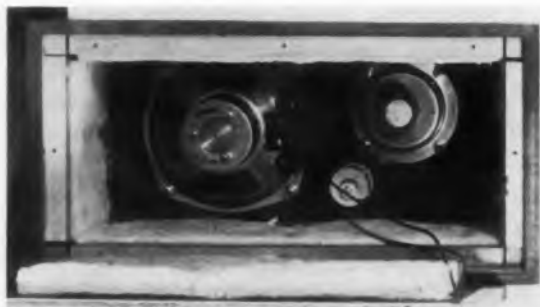
This compact bookshelf GE unit is a two way system. Back is removed to show 6" woofer at left, 2 3/4" tweeter at right, and crossover network between. Assembled cost is $50 complete. Kit price is $30.
