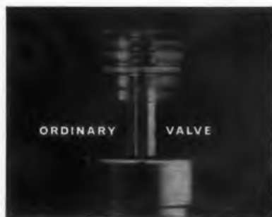
Test reveals that ordinary valve piston bounces four (sometimes six) times . . . the first two great enough to "ghost" the tone.
