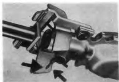
Typical phono pickup (crystal type) showing (indicated by two arrows) the replaceable stylus. In this case the stylus is simply pulled out of holder; no screws are involved. (Courtesy Jensen)
