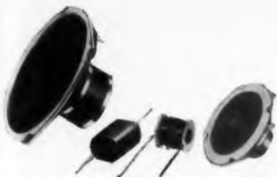
G.E. two-way speaker system before mounting in baffle. Left is heavy woofer, right cone tweeter, middle units are crossover. Total cost: $29.95.
