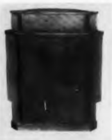
Wharfedale C-500 sand-filled corner enclosure. Not a corner horn, despite appearance. Corner placement produces more sound output than placement along a wall. Small vents at bottom left and right act somewhat like a bass reflex port. Model C-500 costs $180. Similar model with less finely-finished wood is $115. Both prices are exclusive of drivers.
