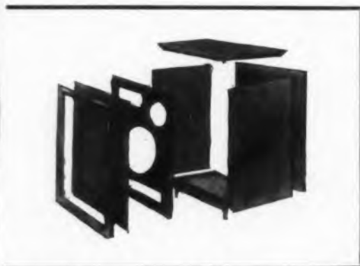
Typical bass reflex kit shown in exploded view. Bottom slot is bass reflex port. Large circle mounts 12-inch speaker. Small hole is for mid-range cone. Upper left hole takes horn tweeter. Holes not used at first are covered with wood pieces. Allied Radio Corp. Fig. 4.
