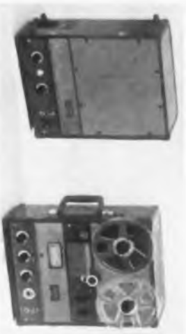
Ampex 601 recorder-playback runs at 7 1/2 ips, records mono, plays back stereo or mono tapes through companion speaker-amplifier at left, Model 620.
