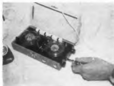
Miniature recorders are capable of high quality pickup when a high quality microphone is used. At top is the Mahawk Midgetape 500 which records at 3\frac{3}{4} ips, has recording meter and uses special 15-minute (times 2 tracks) cartridges. Costs $265. Lower photograph shows Fi-Cord, which uses standard 3-inch reels, records at 7\frac{1}{2} or 1\frac{7}{8} ips, includes small monitor speaker. Recorder costs $290.
