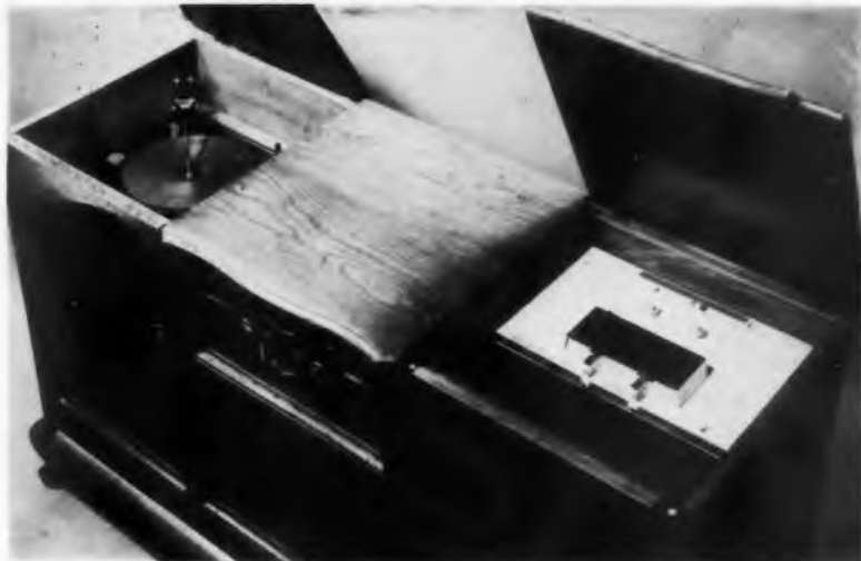
One of the most important recent developments is the new line of tape players by Bell Sound. The mechanism shown at left in the console above handles the RCA slow-speed (3 1/4 inches a second) four-track magazine tape recording. Bell is supplying the mechanism six different ways, from the mechanical unit, for playing through any stereo high fidelity preamplifier-amplifier, to complete systems, including amplifiers and speakers. The cost of the players is about $100 more than that of associated parts. RCA also is finally delivering its tape players. The quality is surprisingly good. The phonograph record changer in console above is Garrard RC 88.
