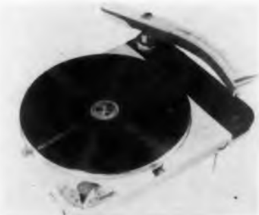
Thorens TD-124, four-speed turntable has modified belt-drive and massive 11 1/2-pound turntable. Speed is adjustable for exact pitch. Dark section at right is wood for mounting any tone arm. Shown here is Fairchild 280 arm. Built-in neon light and mirror shows when exact speed is set. It costs $99.75, less base.
