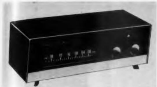
Tuners may be built from kits today because critical parts are pre-assembled. Ninety percent of internal wiring is eliminated by use of printed circuit boards. Heathkit FM-4 costs $34.95.
