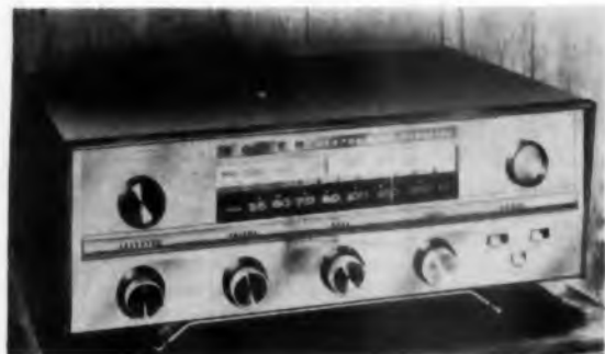
Bogen SRB-20 is a complete receiver, much like the Fisher 600 shown here also. Two 10-watt amplifiers and complete controls are included, as well as separate FM and AM tuners. The price is $199.50.
