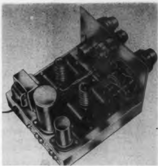
Lafayette Radio has a kit for stereo control of any two power amplifiers. This unit can go at a great distance from other electronics, near listening position. Printed circuit board simplifies wiring of this kit.
