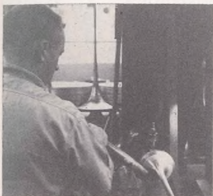
6. The crude bells seen in the previous photo are worked up into something approximating the final shape, then spun on a lathe, as seen here.
