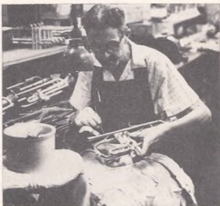
9. The various parts of horns—valves in their casings, tubing, bells—wait on a workman's bench. He assembles the standardized parts.
