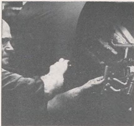
2. The mechanical heart of a trumpet is the valve pistons. A machine, working to exceptionally fine tolerances produces them. Here, a workman removes one.
