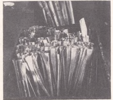
5. Now the bell of the trumpet. Flat sheets of brass are doubled over to form crude bell shapes, a bin of which are seen in this photograph.
