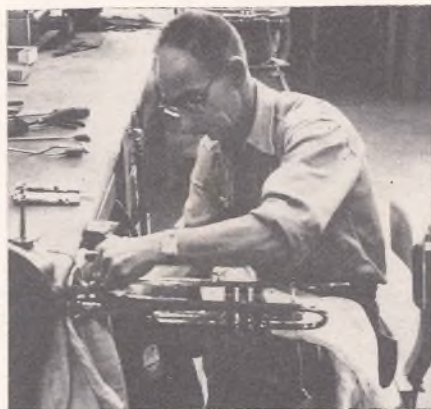
10. Still largely a hand art—you'll see a workman holding up a horn to check its alignment by eye — instrument assembly is the crucial stage. Silver solder is used.
