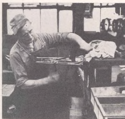
12. Final polishing. Each individual valve casing, as well as more accessible parts of the horn, is given a finishing touch by hand polishing.
