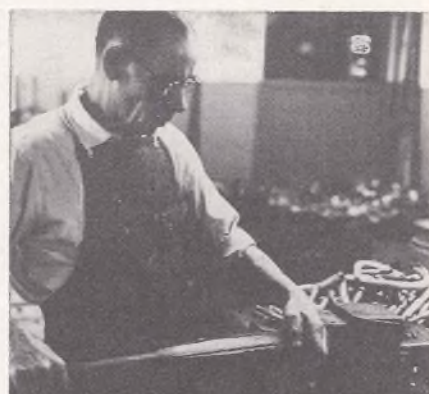
8. How do they bend the brass tubing so that it doesn't buckle in the process? They fill them with molten pitch, let it harden, then bend them to shape, as this man is doing.
