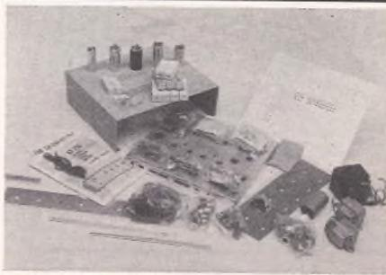
All parts of Lafayette stereo amplifier KT-250 spread out. Note instruction manual and line cord at left.
