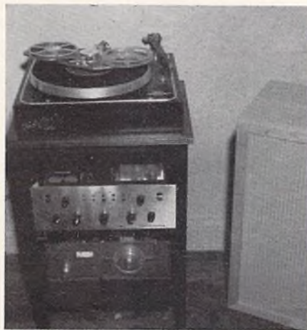
Complete stereo home music center—Tape, FM, phonograph. AR-3 speaker at right is balanced by second speaker eight feet to left. The components turntable is shown with Gramdeck tape attachment in place. The tape head plays through Madison-Fielding dual-20 watt stereo amplifier. At bottom is Scott 310-C FM tuner. Arm and cartridge are by Pickering.
