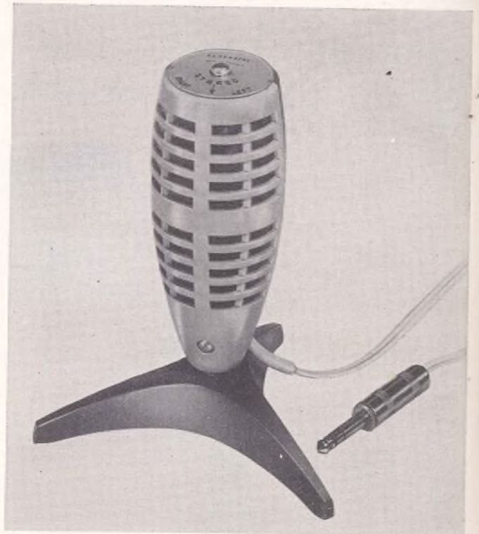
Stereo microphone for use with home and semiprofessional recorders has two microphones in one. Using famed M-S system long employed on the Continent, internal mike elements face performers 45 degrees from each other and pick up sounds from opposite sides of groups. It costs $39.50 and is standard equipment with Norelco stereo 400 recorder.
