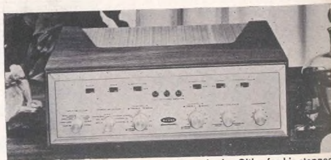
All-in-one stereo Scott amplifier was chosen by Ira Gitler for his stepped-up high fidelity system. Separate bass and treble controls for each channel allow compensation for unlike stereo speakers. Other controls include rumble and scratch filters, speaker-swapping switch, and two switchable magnetic phono inputs. Dual 12-watt Model 1222, excluding case, costs $139.
