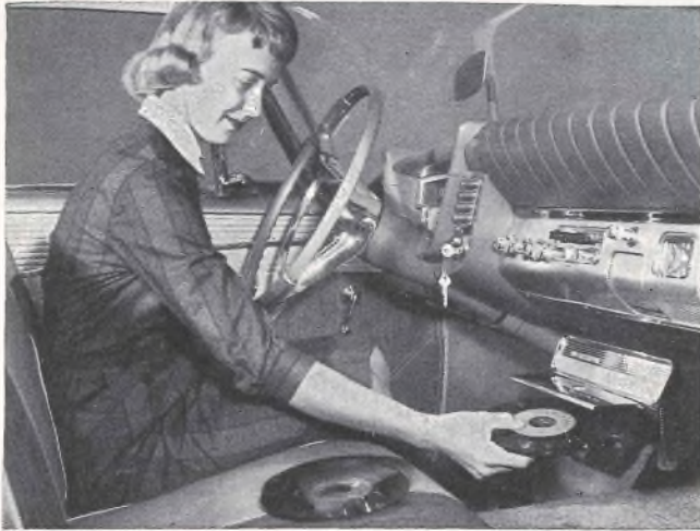
Loading a stack of 45-rpm discs into the RCA-Chrysler auto phonograph is as easy as it looks. Discs are pushed into place, lid pushed down, and start button pressed. It costs $120 at Plymouth-DeSoto dealers. Player works through car radio.
